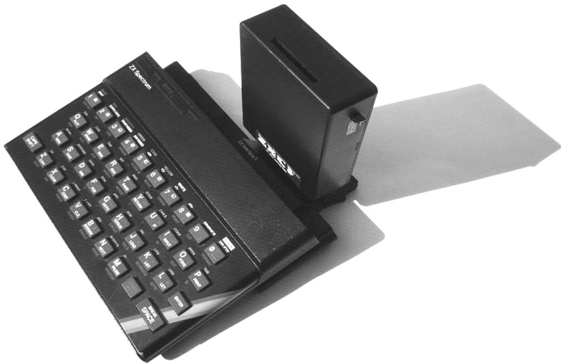
Fig 7.3 Sami Vehmaa's ZXCF compact flash interface – attached here to a rubber-keyed Spectrum via an IF 1 – is emulated by Fuse.
